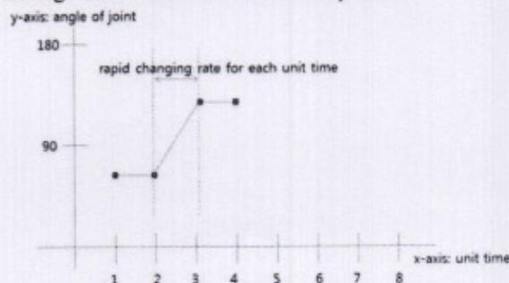
Fig. 3. Straight line-type joint trajectory
