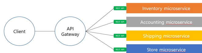
Figure 4. Micro service integration based on API-Gateway style
