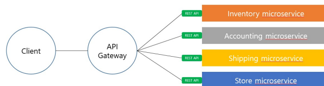
Figure 4. Micro service integration based on API-Gateway style
