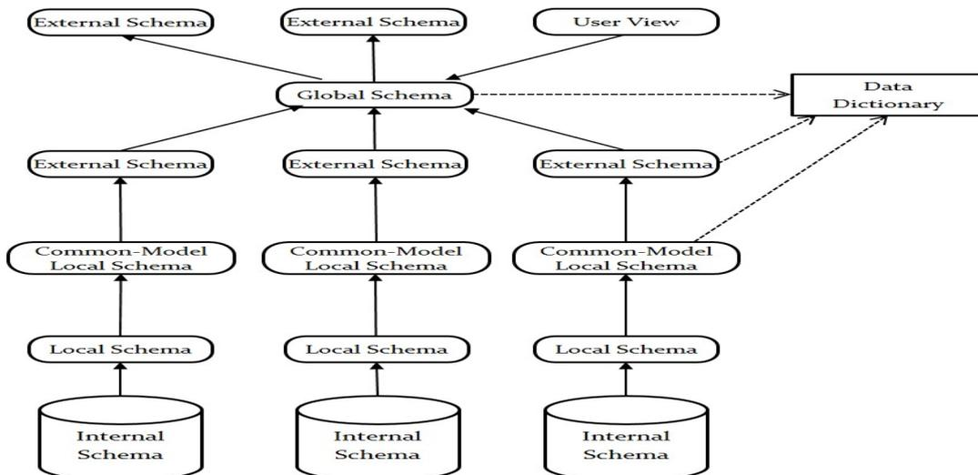
Figure 5 The architecture method for FDBS development
