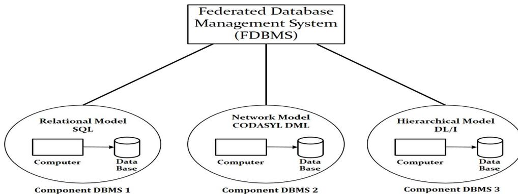
Figure 1 Federated database management system and its components
