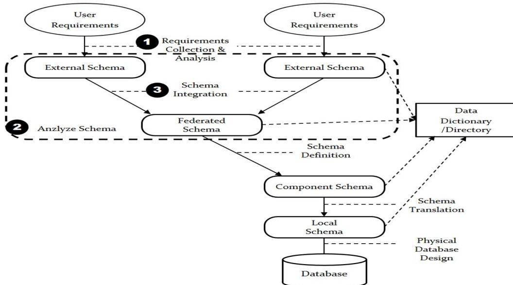
Figure 4 Top-down FDBS developing process
