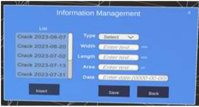
Fig. 7. Crack information edit panel
